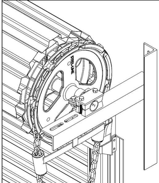
5. Fit chain lock onto the wall.
