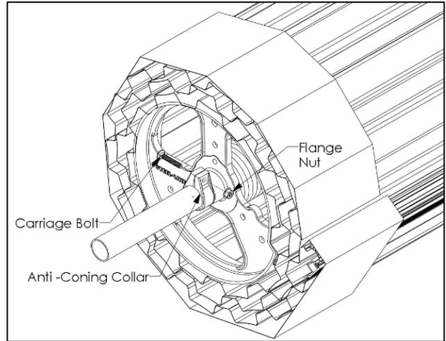
4. Check if shaft length has no interferences and fits within the side clearances. Trim the shaft if necessary.
