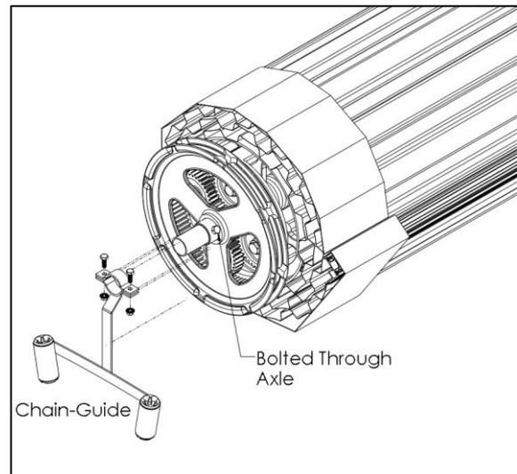
1. Line up and fit the ring gear with provided bolts and nyloc nuts to drum.
