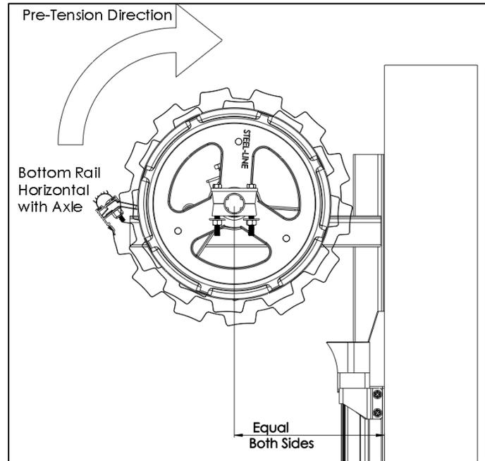
6. While holding the wrapped curtain, carefully cut and remove the packaging and slowly pull the curtain into the guides, removing any cardboard and tape.
