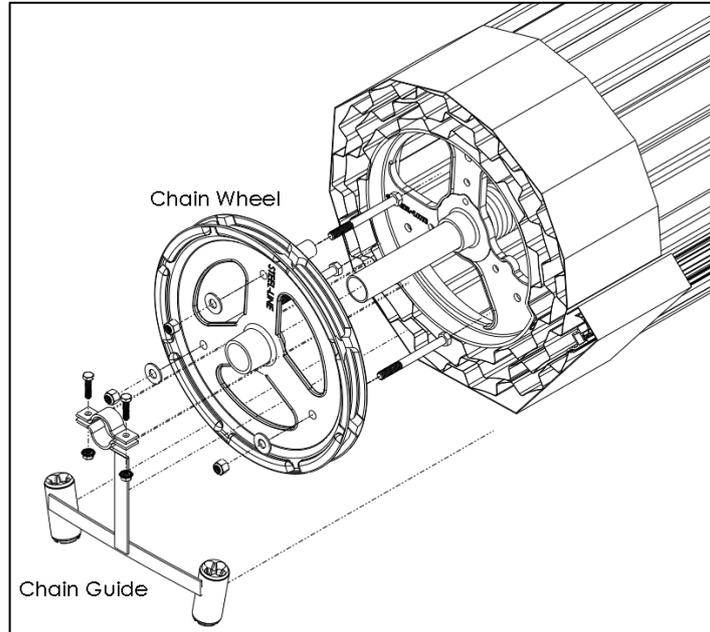
1. Line up the chain wheel with the drum wheel on the drive side and secure with bolts and nyloc nuts provided.
