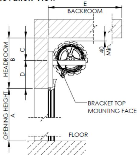
For curtain widths 3100 to 5500mm
