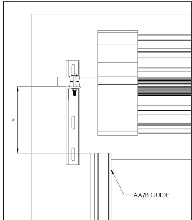
2. Fix the nylon lead-in to the top of the guide with the provided 8G-18x1½" self-tapping screw.
