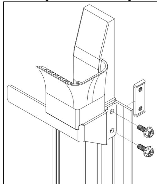
5. Fix the guide to the substrate through the top and bottom slots loosely.
