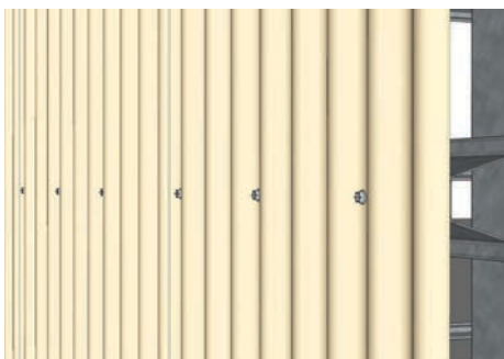
Screws as per wall sheeting profile
