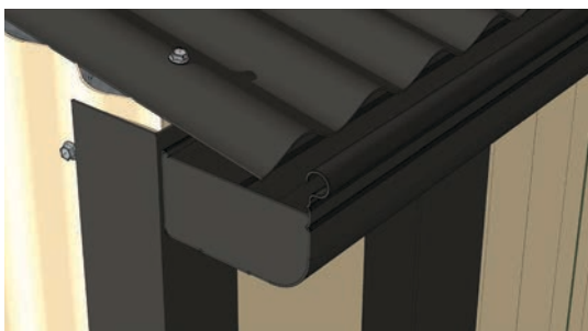
Overhang gutter by approx. 50mm
